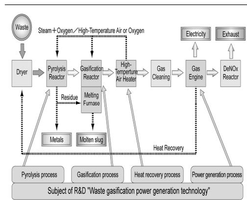
Fig. 1 Development of high efficient waste pyrolysis and gasification typed WTE
