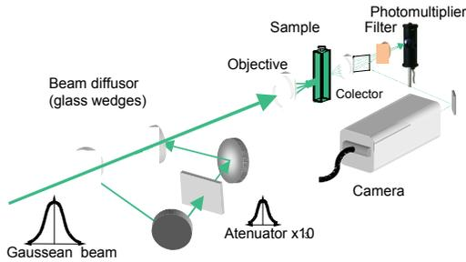
Fig. 1. Experimental set-up for a cylinder-shape photo-bleaching.
