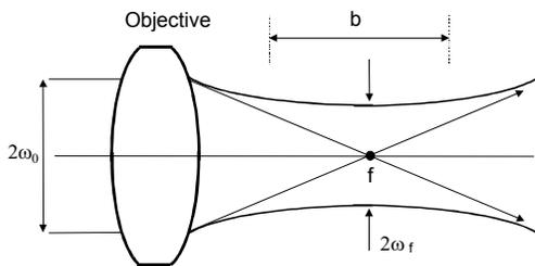
Fig. 2. Detail of the beam after trespassing the objective.
