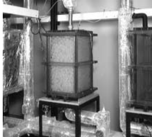
Fig.2. Prototype of encapsulated ice system.
