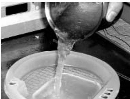
Fig.4. Ice-water slurry with fluidity (IPF=20%).
