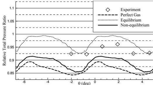
Fig. 8. Exit relative total pressures at 35% span.
