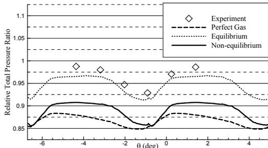
Fig. 10. Exit relative total pressures at 55% span.
