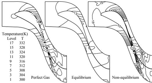
Fig. 4. Temperature distributions at 50% span.
