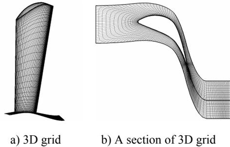
Fig. 1. The sketch of computational grid.
