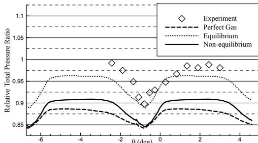
Fig. 11. Exit relative total pressures at 65% span.
