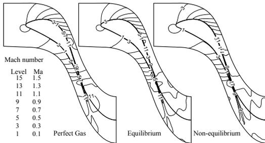
Fig. 5. Mach number distributions at 50% span.
