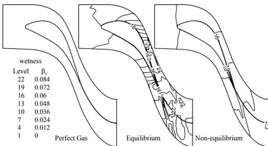
Fig. 6. Wetness distributions at 50% span.
