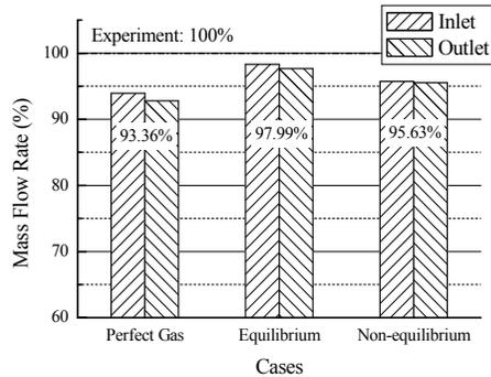
Fig. 7. Comparison of relative mass flow rate between numerical results and test data.
