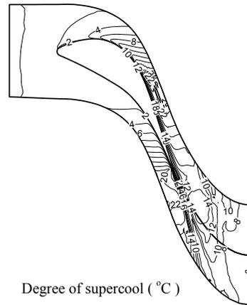
Fig. 2. Distribution of supercooling at 50% span.
