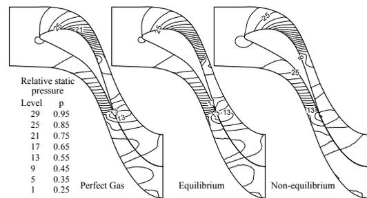
Fig. 3. Relative static pressure distributions at 50% span.
