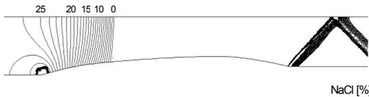
Fig. 3. Saturation concentration of NaCl [%] in SSZ droplets in the nozzle.
