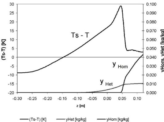
Fig. 8. Subcooling  $(Ts - T)$ , heterogeneous wetness  $y_{\text{Het}}$ , homogeneous wetness  $y_{\text{Hom}}$  along nozzle straight wall.
