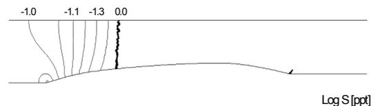
Fig. 2. Solubility (Log S [ppt]) of NaCl in superheated water steam in the nozzle.
