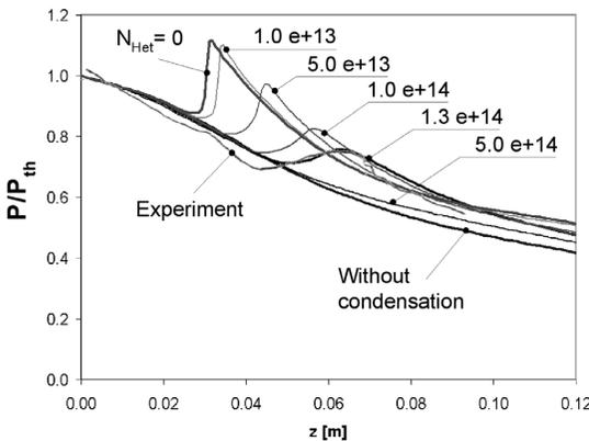
Fig. 4. Relative pressure  $P/P_{th}$  along the straight wall of divergent nozzle part,  $R_{Het} = 1.0 \text{ e-}8 \text{ m}$ .
