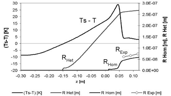
Fig. 9. Subcooling  $(Ts - T)$ , heterogeneous droplet radius  $R_{\text{Het}}$ , homogeneous droplet radius  $R_{\text{Hom}}$ , experiment  $R_{\text{Exp}}$  along the nozzle straight wall.
