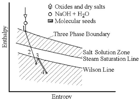
Fig. 1. Steam expansion line in phase transition zone.
