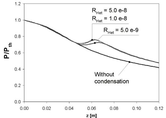
Fig. 5. Relative pressure  $P/P_{th}$  along the straight wall of divergent nozzle part,  $N_{Het} = 1.3 \text{ e+}14 \text{ kg}^{-1}$ .
