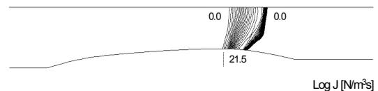
Fig. 6. Spontaneous nucleation rate ( $\text{Log J} [\text{Nm}^{-3} \text{ s}^{-1}]$ ) in the nozzle.
