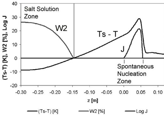
Fig. 7. Concentration of NaCl in droplets of SSZ  $W_2$ , spontaneous nucleation rate  $J$ , subcooling  $(Ts - T)$  along the nozzle straight wall.
