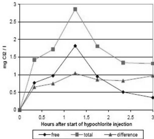
Figure 9: chlorine measured- hypochlorite injection of 01/07/03 (conditioning with polyaspartate)
