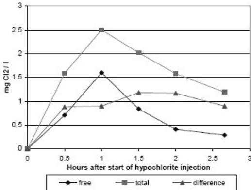
Figure 8: chlorine measured- hypochlorite injection of 03/06/03 (conditioning with polyacrylate)
