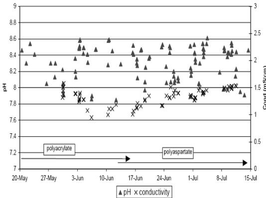
Figure 6: pH and conductivity of the circulating water
