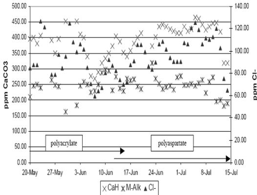
Figure 5: calcium hardness, chlorides and M-alkalinity in the circulating water (daily average)
