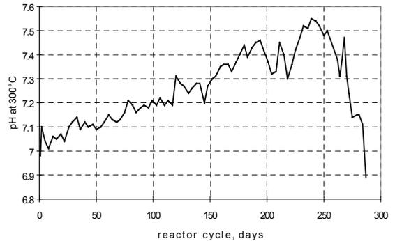
Fig. 2 Typical  $pH_{300}$  course during the reactor cycle for standard water chemistry (VVER-440 unit)
