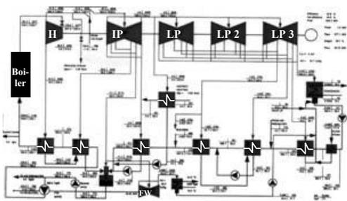
Fig. 1. The water-steam circuit of ASV5.
