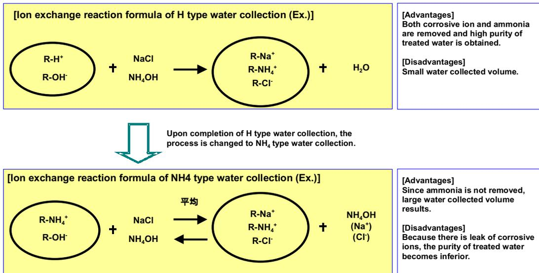
Fig. 7 Water collecting system and features of condensate demineralizer
