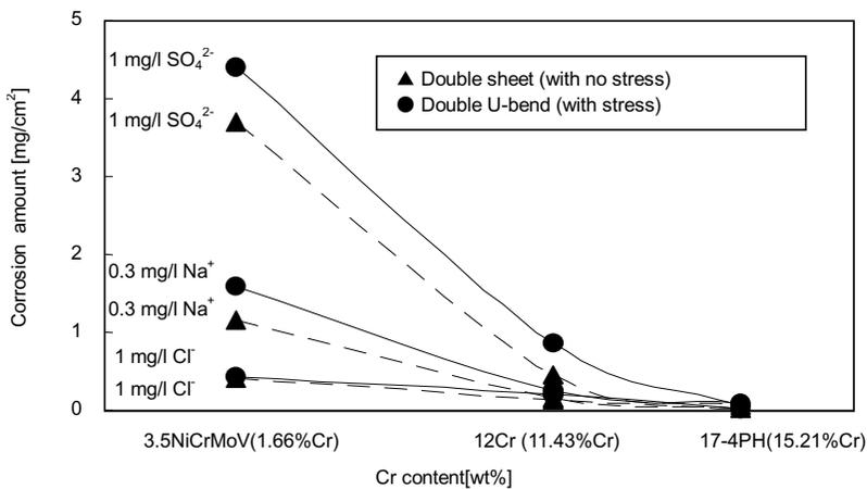
Fig. 5 Relation between corrosion rate and Cr content
