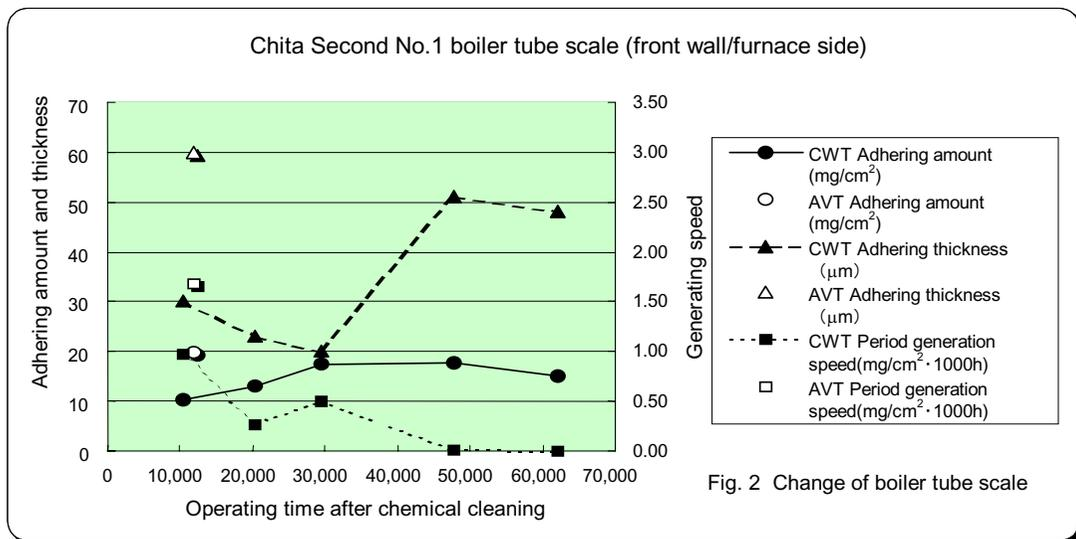
Fig. 2 Change of boiler tube scale
