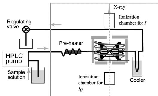
Fig. 4. Schematic drawing of a system for the EXAFS measurement.
