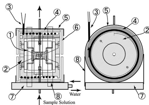
Fig. 3. Schematic drawings (side cross section and front view) of a heating system of the high pressure optical cell. ① High pressure optical cell. ② Heating jacket. ③ Sheathed heater. ④ Rock wool. ⑤ Stainless steel container. ⑥ Heat insulator. ⑦ Stage. ⑧ Band. In the front view, the heat insulator is omitted.
