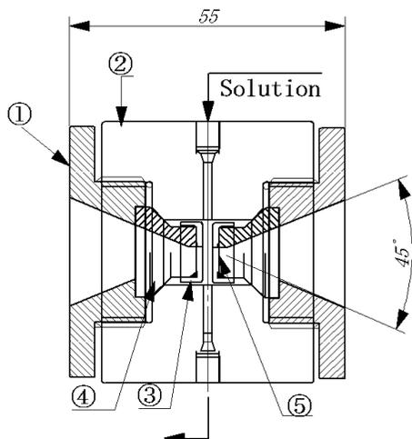
Fig. 1. Cross section of a high-pressure and high-temperature optical cell. ① Window support screw. ② Cell body. ③ Window screw cap. ④ Window support. ⑤ Diamond window.
