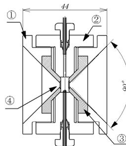
Fig. 2. Cross section of a wider aperture high-pressure and high-temperature optical cell. ① Window support screw. ② Cell body. ③ Window support. ④ Diamond window.
