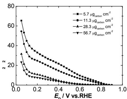
Fig. 7. The ratio of  $\text{H}_2\text{O}_2$  formation upon oxygen reduction at 20 wt% Pt/C ( $56.7$ ,  $28.3$ ,  $11.3$ , and  $5.7 \mu\text{g} \text{cm}^{-2}$ ) loaded on GC in  $1 \text{ M HClO}_4$ .
