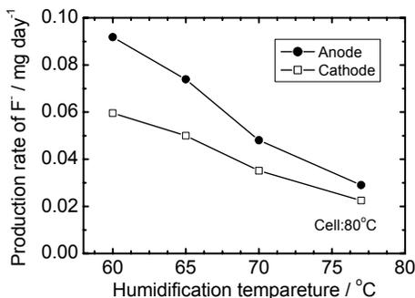
Fig. 13. Effect of humidification temperature on the production rates of fluoride ion during OCV durability test. MEA: 25 cm<sup>2</sup>, Cell temp: 80°C, Atmospheric pressure, H<sub>2</sub>/Air = 150/150 mL min<sup>-1</sup>.
