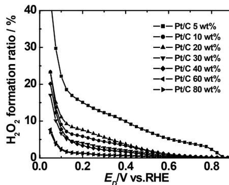
Fig. 5. The ratio of H<sub>2</sub>O<sub>2</sub> formation upon ORR at 5-80 wt% Pt/C (56.7 μg<sub>carbon</sub> cm<sup>2</sup>) loaded on GC in 1 M HClO<sub>4</sub>.
