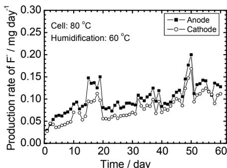
Fig. 12. Production rates of fluoride ion in condensed water from the anode and cathode during OCV durability test. MEA: 25 cm<sup>2</sup>, Cell temp: 80°C, humidification: 60°C, Atmospheric pressure, H<sub>2</sub>/Air = 150/150 mL min<sup>-1</sup>.
