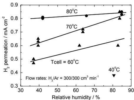
Fig. 8. Effect of cell temperature and humidification on  $\text{H}_2$  crossover current. Atmospheric pressure,  $\text{H}_2/\text{Ar} = 300/300 \text{ mL min}^{-1}$ .
