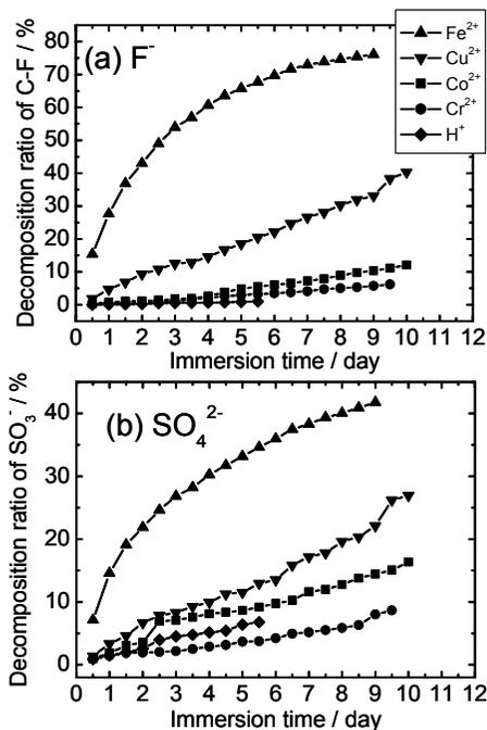
Fig. 2. Decomposition ratios of (a) C-F bonds and (b) sulfonic acid moieties of Nafion after durability test in 30%  $\text{H}_2\text{O}_2$  at  $80^\circ\text{C}$ .
