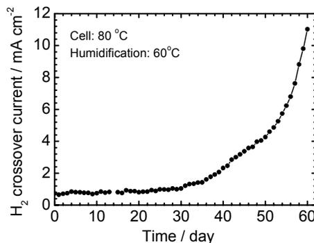
Fig. 11. Variation of  $\text{H}_2$  crossover current during OCV durability test. MEA:  $25 \text{ cm}^2$ , Cell temp:  $80^\circ\text{C}$ , humidification:  $60^\circ\text{C}$ , Atmospheric pressure,  $\text{H}_2/\text{Air} = 150/150 \text{ mL min}^{-1}$ .
