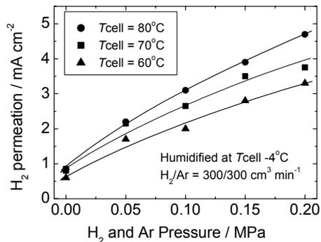
Fig. 9. Effect of gas pressure on  $\text{H}_2$  crossover current.  $P_{\text{H}_2} = P_{\text{Ar}}$ ,  $\text{H}_2/\text{Ar} = 300/300 \text{ mL min}^{-1}$ .
