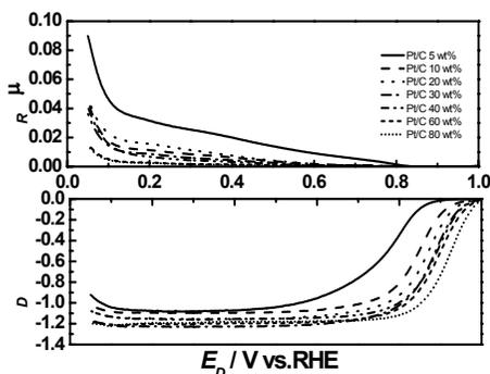
Fig. 4. Hydrodynamic voltammograms for oxygen reduction in 1 M HClO<sub>4</sub>. Disk electrodes: 5-80 wt% Pt/C (56.7 μg<sub>carbon</sub> cm<sup>2</sup>) loaded on GC, Ring electrode: Pt. Rotating rate: 900 rpm.
