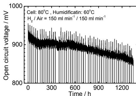
Fig. 10. Variation of OCV during OCV durability test. MEA:  $25 \text{ cm}^2$ , Cell temp:  $80^\circ\text{C}$ , humidification:  $60^\circ\text{C}$ , Atmospheric pressure,  $\text{H}_2/\text{Air} = 150/150 \text{ mL min}^{-1}$ .
