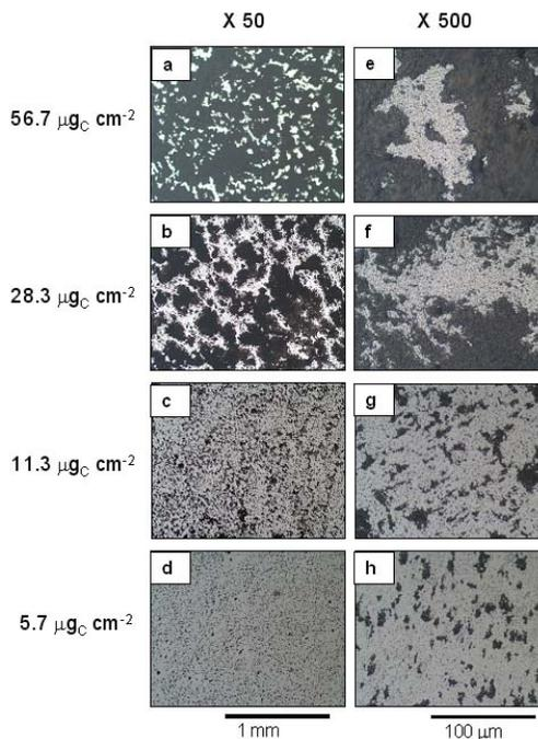
Fig. 6. Optical micrographs of 20 wt% Pt/C dispersed on GC. Pt/C loadings: (a, e) 56.7, (b, f) 28.3, (c, g) 11.3, and (d, h) 5.7 μg cm<sup>-2</sup>.
