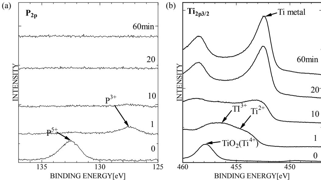
Fig. 3 XPS spectra of anodic oxide film of Ti and P. anodic oxidation at 50V (a) P2p (b) Ti2p3/2
