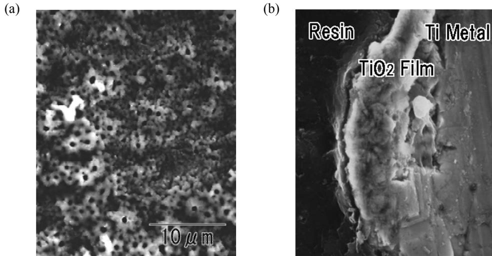
Fig.1 .SEM image of anodic titanium oxide titanium films.
