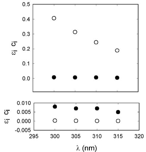
Fig. 3. A typical experiment at 423 K showing the contribution to optical absorption of different copper species. Solid circles correspond to  $\text{Cu}^{2+}(\text{aq})$  ions, open circles in upper panel:  $\text{CuSO}_4$  ion pair, lower panel:  $\text{CuOH}^+$ . Note the different scale of the ordinates in the two graphs.
